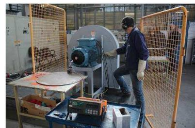
Checking the vibration of the unit. In this case only 1.5mm/s rms; which is a low vibration level.
